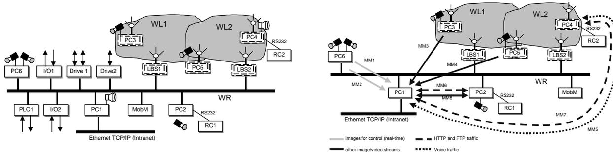
Fig. 3. RFieldbus network topology (left), Multimedia streams (right)
