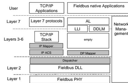
Fig. 1. PROFIBUS and TCP/IP integration
