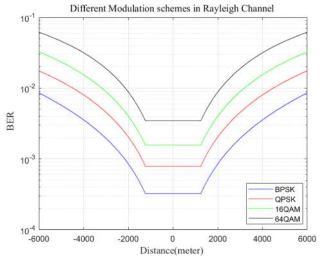
**Figure 6:** BER vs. distance of different modulation schemes in Rayleigh channel.
