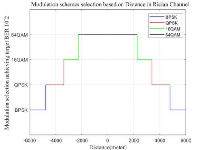
**Figure 11:** Illustration of distance-based selection of various modulation schemes in Rician channel.**Table 6:** Illustration of switching threshold values of distance and SINR for various modulation schemes in AWGN, Rayleigh and Rician channels.
