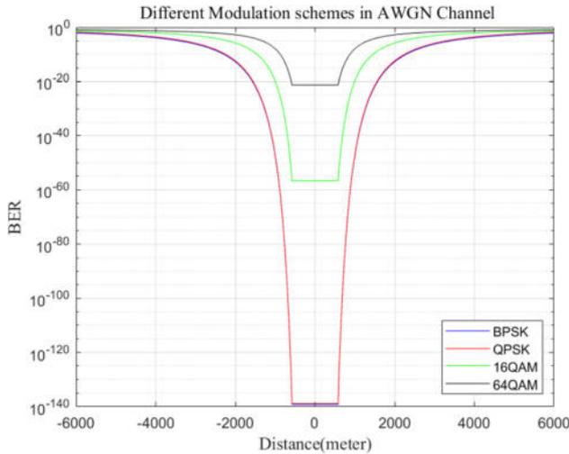
Figure 3: BER vs. distance of different modulation schemes in AWGN channel.
