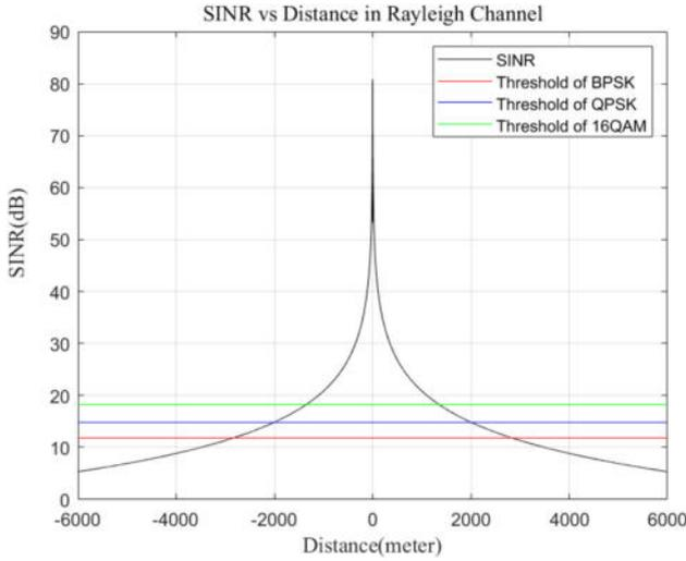
Figure 7: SINR vs. distance in Rayleigh channel.
