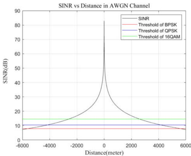
Figure 4: SINR vs. distance in AWGN channel.
