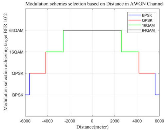
**Figure 5:** Illustration of distance-based selection of various modulation schemes in AWGN channel.
