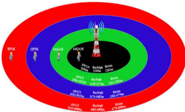
Figure 12: Illustration of distance-based selection of various modulation schemes in AWGN, Rayleigh and Rician channels.
