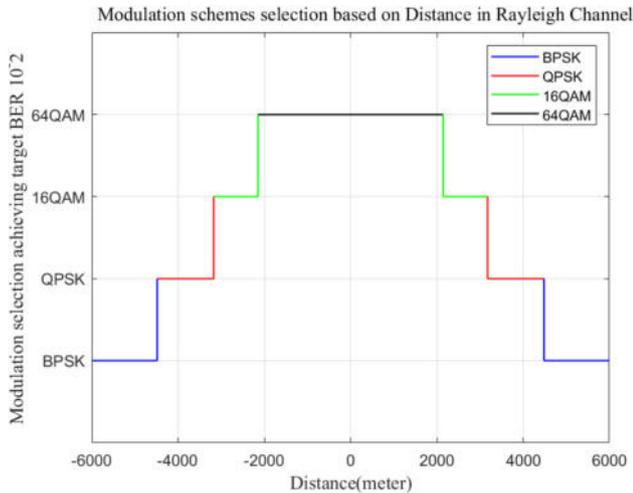
**Figure 8:** Illustration of distance-based selection of various modulation schemes in Rayleigh channel.
