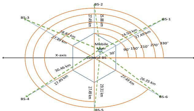
**Figure 2:** Illustration of distance and angle between co-channel BSs and central BS and distance between mobile user and co-channel BSs.
