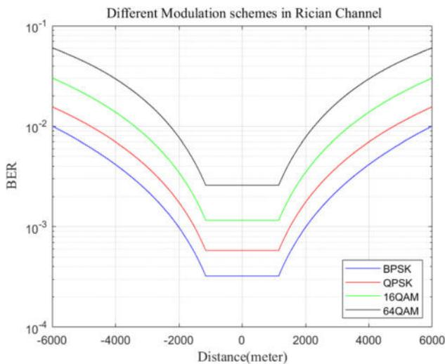
**Figure 9:** BER vs. distance of different modulation schemes in Rician channel.
