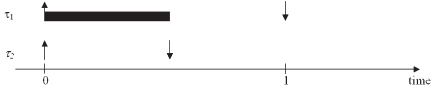
Figure 1: A task set where SM misses a deadline and the utilization is 50%. An arrow pointing upwards indicate the arrival of a task. An arrow pointing downwards indicate the deadline of a task.
