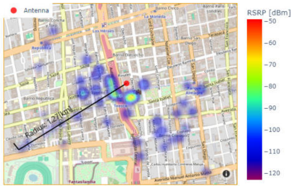
Fig. 3. RSRP measurement campaign conducted in a central neighborhood in Santiago, Chile. Latitude and longitude of the NB-IoT base station: -33.451392, -70.657928.
