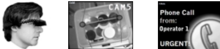
Fig. 5. The TekGear M1 HMD (left). Views at the HMD: camera view (centre); phone call (right)
