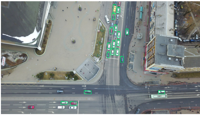
Fig. 15: Example of Faster R-CNN misclassifications on an image of the PSU dataset, showing several false negatives (non detected cars).
